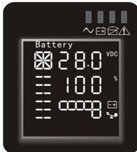
Press and hold the inquiring button
