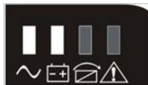
When the utility power is not available or is not stable, UPS will turn to battery mode immediately. Continuously working on battery mode can last for 20 hours depending on the battery volume and the load. If battery discharge for 20 hours and the load is lower than 10% of rated power, the UPS will alarm for ½ hour and then shutdown to protect the batteries.
