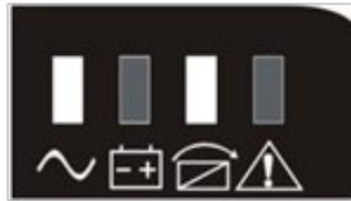
When the input utility equals the input range of the ECO mode and the ECO function is activated, the UPS will operate in ECO mode. If input AC utility exceeds the range of ECO several times in a row in a minute but stays in the inverter input range, the UPS will operate on inverter mode automatically.
