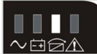
Bypass yellow LED is on, the buzzer beeps once every 2 minutes. The warning red LED is on when beeping. LCD displays are according to the exact load and battery capacity.
