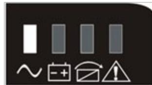
When input AC utility is in line with the working conditions, UPS will work in line mode.
