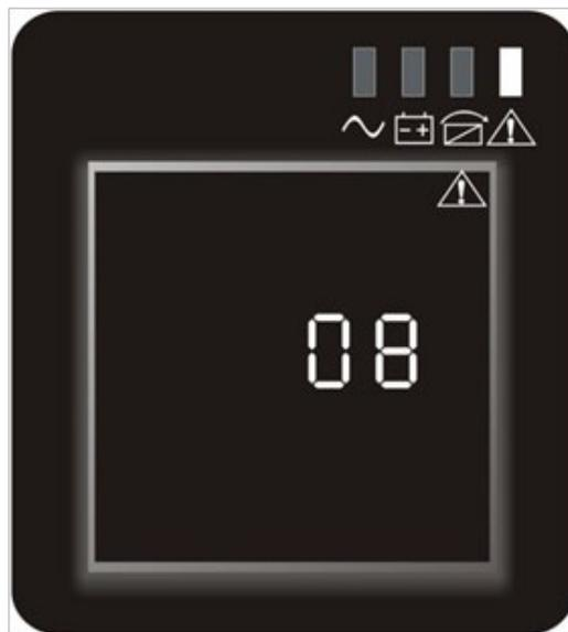
**Fault mode (LCD interface with the fault code display)**
