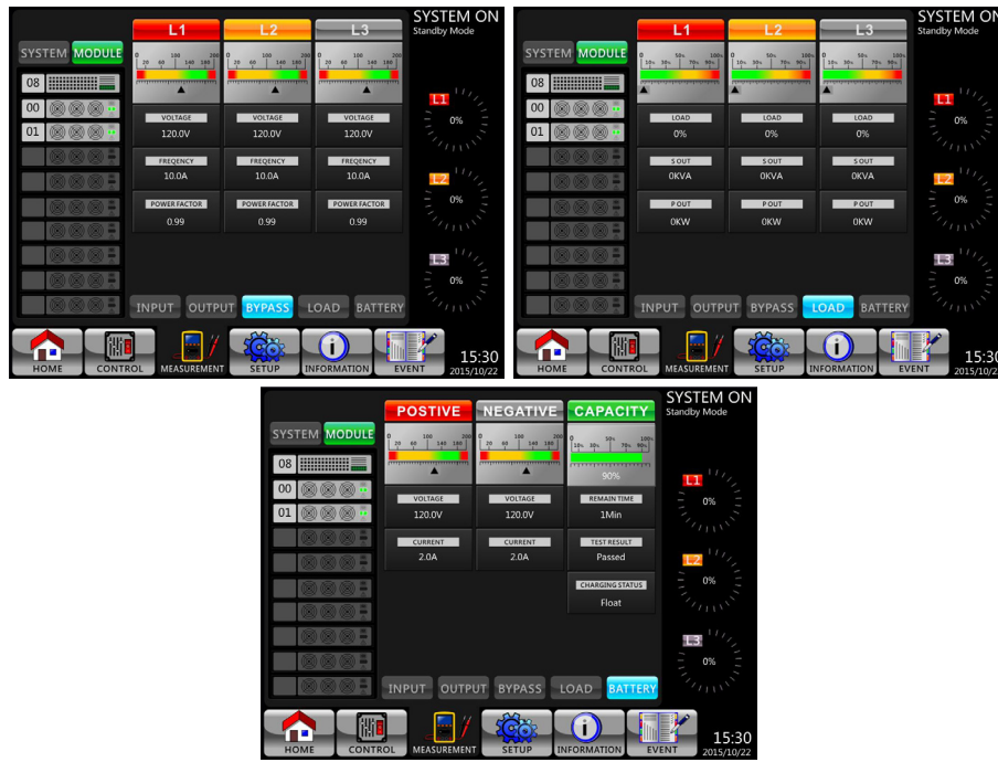
Figure 4-10 Module Measurement Screens
