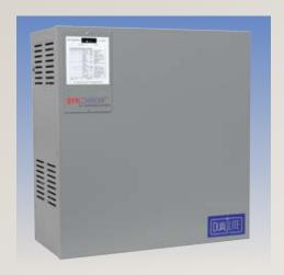
In 2005, Dual-Lite introduced the **Synchron Central Lighting Inverter System**, with output ratings from 400 VA to 2100 VA, and without the myriad user control features and self-test/self-diagnostic circuitry of the Spectron LSN unit. This design again utilized a digital circuitry approach employing topography identical to the Spectron LSN system, but using field effect transistors (FETs) instead of IGBTs due to the lower output ratings. The Synchron series is still in production today.
