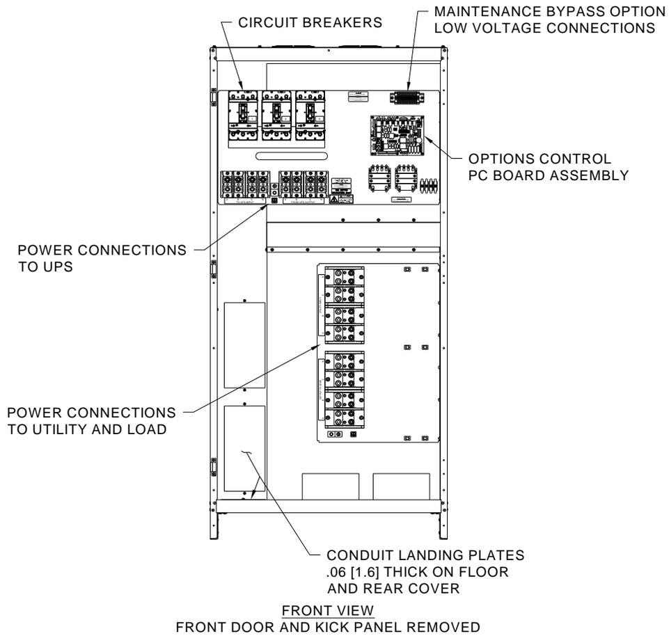
**Figure 4 - Inside Front View of Transformer Cabinet**
