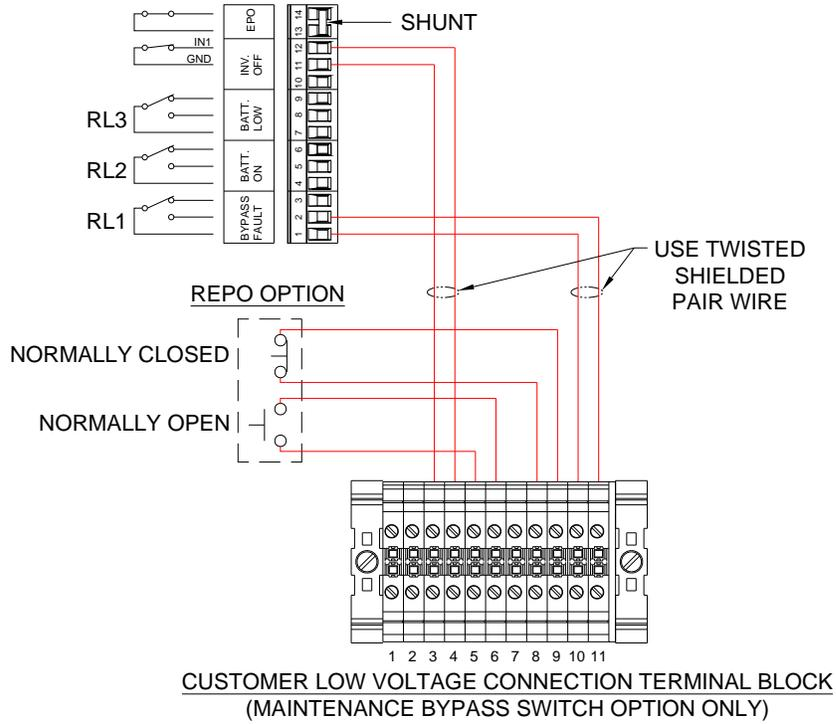
**Figure 7 - Customer Low Voltage Connection Terminal Block**
